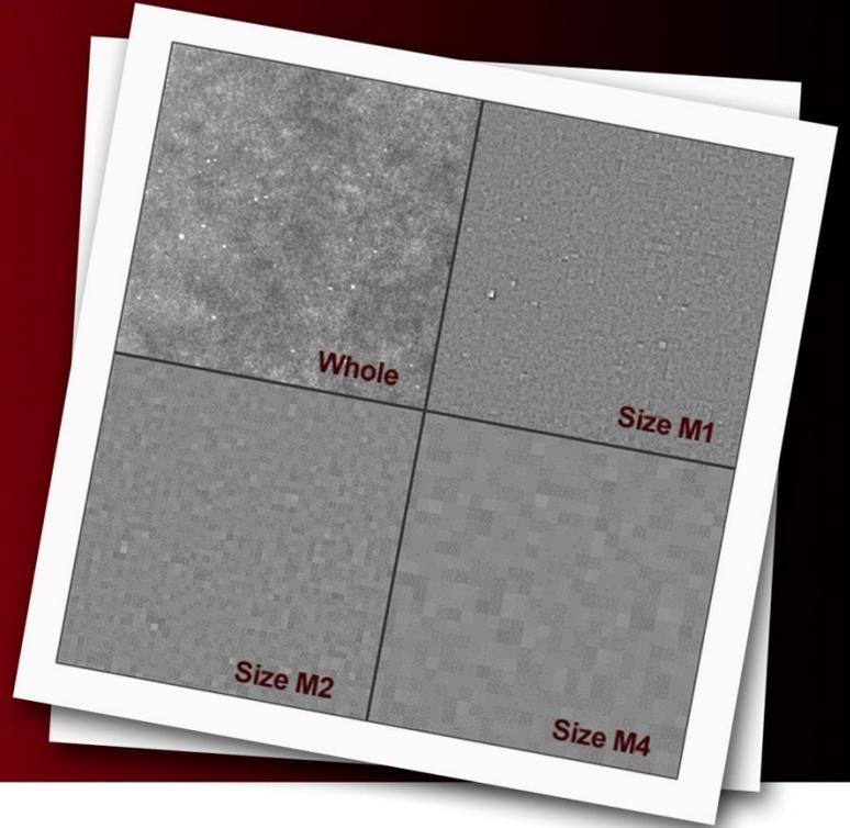
***The OMA uses a wavelet-based technique that partitions print/coating mottle into its size components.***
